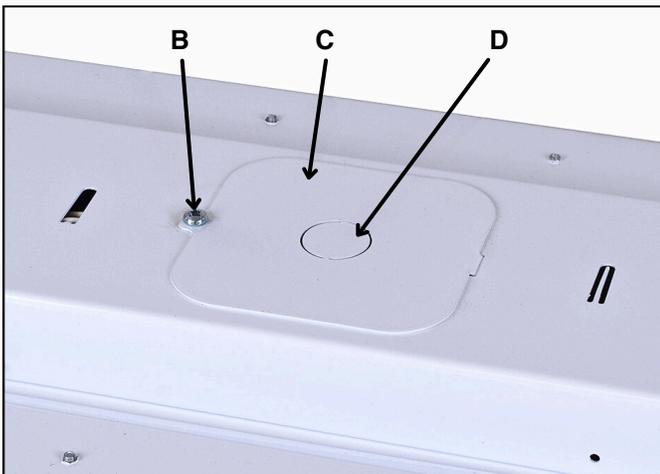
5. If incoming power supply is household romex wire, install appropriate wire coupler/clamp (not included) into housing where knockout plug was removed.
