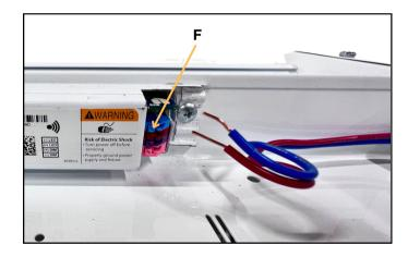
**3.** Once the buttons are pressed, gently pull all of the wires away from the driver to fully disconnect them. Take note of the wire locations for easier reinstallation later.
