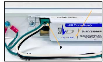
Using a small tool, gently push the release buttons (F) while holding the wire. This will disengage the wire from the driver socket, allowing removal.
