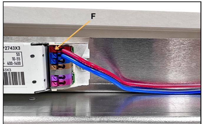
3. Using a small tool, gently push the release buttons (F) while holding the wire. This will disengage the wire from the driver socket, allowing removal.
