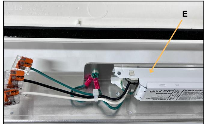
2. On both ends of the driver, locate the wiring connections on the LED boards and ground. To disconnect the wires from the driver, find the small release buttons located on the top of the connection points (F).
